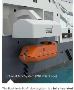
The Boat-In-A-Box™ davit system is a **fully insulated** and air heated closed box performing to **-20 degrees** celcius. Fully operational during ESD and capable of withstanding any extreme weather conditions.
