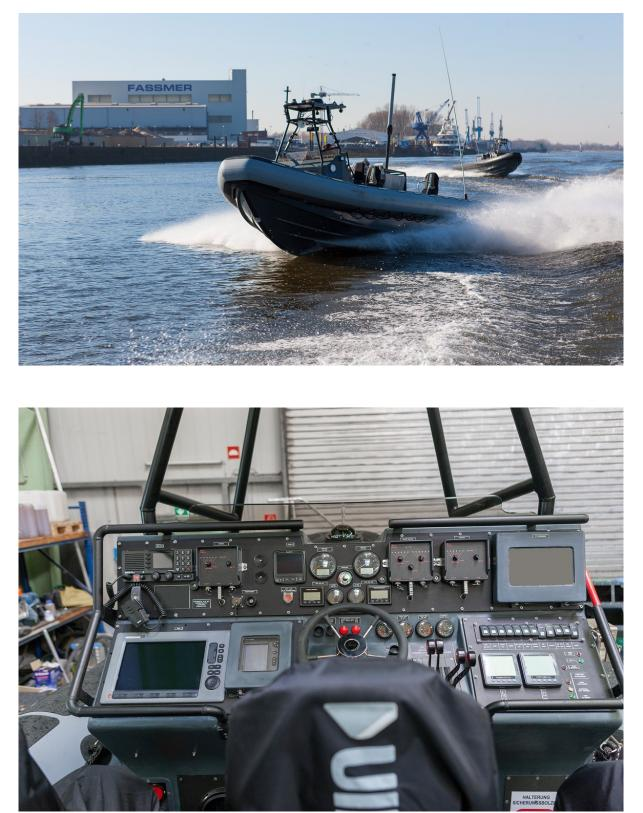
Fully equipped steering console with additional systems according to customers' needs on SFB 10.1
