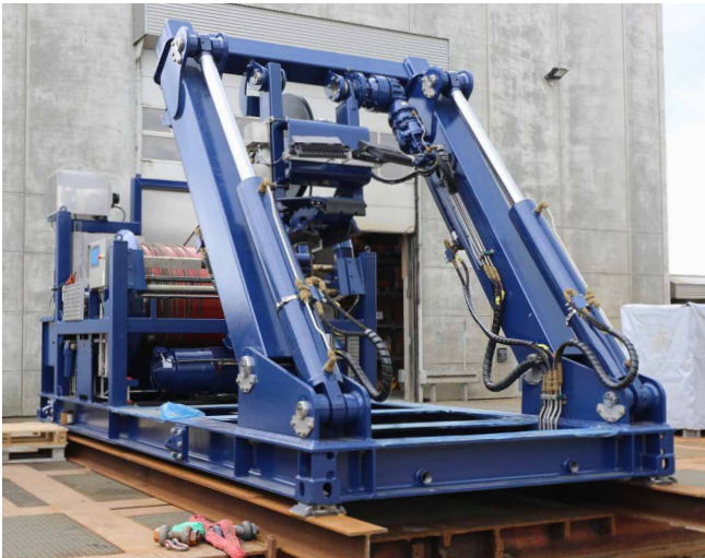
Electrical Compact LARS (Winch and A-Frame). Drum capacity: 3300 meter Ø12.7 mm wire (Optional).
