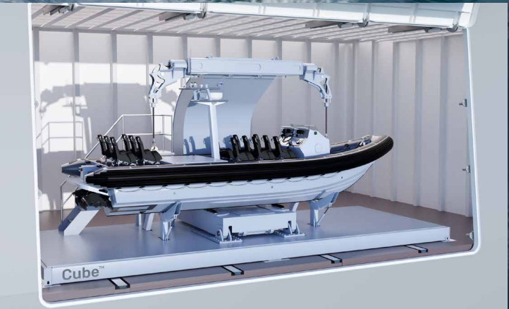
LARS System for probes and towed vehicles placed on a Cube™ Side loader
