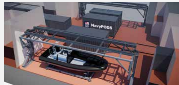
Cube Boat Davit in Mission bay and hangar with Sea State Skidding System
