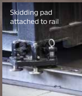
Hydraulic operated skidding dog
