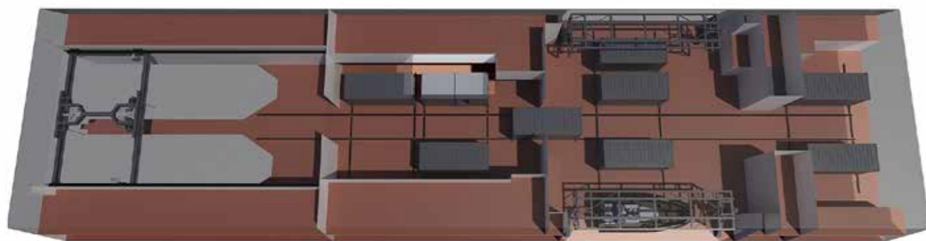
Mission bay and hangar with Sea State Skidding System
