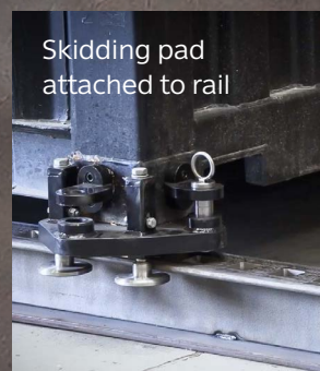
Hydraulic operated skidding dog
